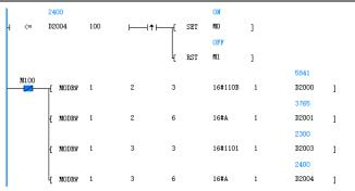
Figure 5.6 Programming case for RS485 communication
